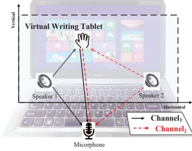
Fig. 1. Illustration of the virtual writing tablet on a laptop.
